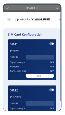
The most important information about the SIM cards can be viewed here. In addition, the SIM PIN of the corresponding card can be stored here.
