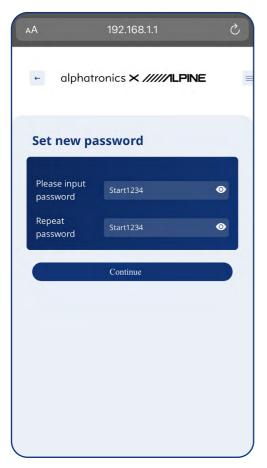
To ensure maximum security for you and your network, the password **must** be replaced with a new one during the initial installation.
