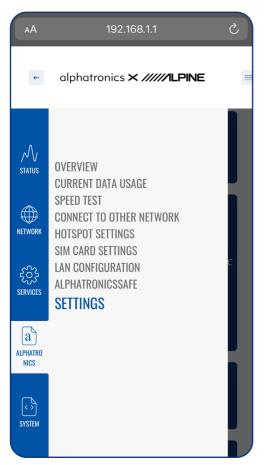
The three dashes at the top right of the logo can be used to open the advanced settings of the unit (professional mode).
