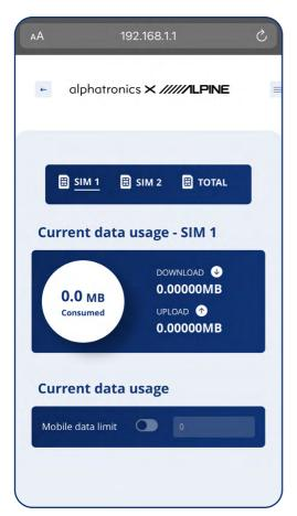
In this level, the data consumption of the respective SIM card can be determined and displayed.
