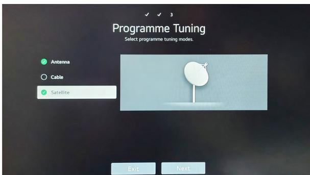
By entering the country beforehand, the system automatically suggests the most frequently used satellite of the country directly. If you would like to enter a different satellite, please select **[other providers]** and confirm with Next.
